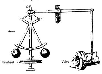
Figure 1 A schematic representation of the governor James Watt designed for his steam engine.
