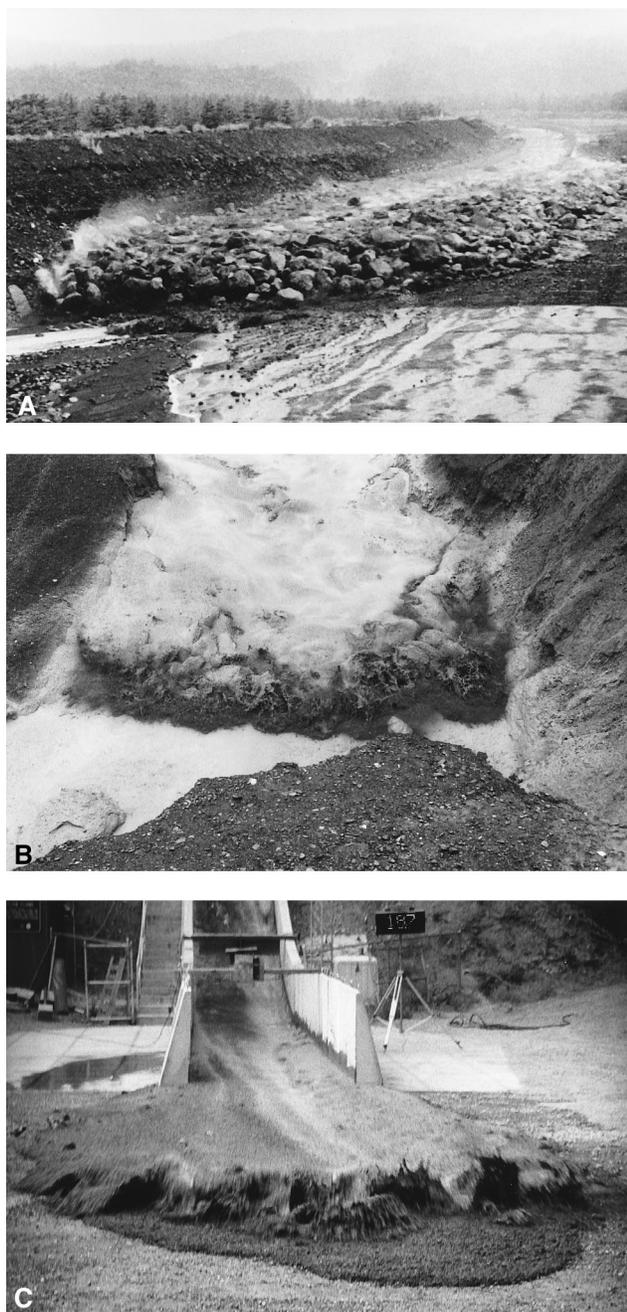
**Figure 8.** Photographs of advancing fronts of debris flow surges. (a) Nojiri River, Kagoshima, Japan, September 10, 1987. Flow is about 20 m wide and 2–3 m deep. (photo courtesy Japan Ministry of Construction.) (b) Jiang Jia Ravine, Yunnan, China, June 24, 1990. Flow is about 12 m wide and 2–3 m deep (photo courtesy K. M. Scott.) (c) USGS debris flow flume, July 20, 1994. Flow is about 4 m wide and 0.2 m deep.
