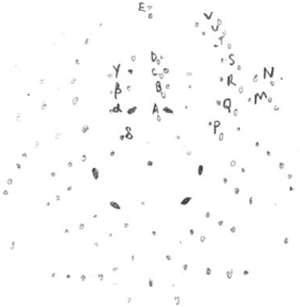
Fig. 2. One of several sets of labeled points made by pricking through the spots on the photograph onto paper and indicating the magnitude of each spot (Royal Institution Bragg MS WLB86, courtesy of the Royal Institution of Great Britain).
