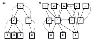
**Figure 24** (a) A typical hierarchical pyramid of control processes with information (dotted arrows) directed toward higher layers and commands directed to lower levels. Sensory inputs are represented by dotted arrows. Arrows and edge-ended lines indicate excitatory and inhibitory control. (b) Heterarchical organization that violates several features of a hierarchical pyramid.
