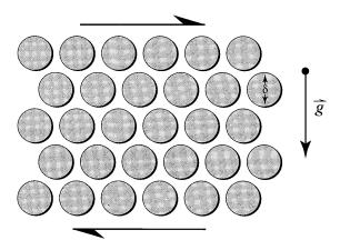
**Figure 14.** Schematic diagram of a steady, uniform, unbounded shear flow of identical solid spheres immersed in a Newtonian fluid. This flow is too simple to represent debris flows, but it provides a basis for assessing scaling parameters that influence stresses.
