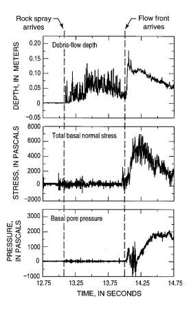
**Figure 10.** Data from Figure 5a plotted on an expanded time base to show details during arrival of the debris flow front. Note that a spray of tumbling rocks precedes the arrival of the flow front, which occurs at  $t \approx 14$  s. Pore pressures do not rise appreciably until the deepest part of the flow front passes the measurement cross section.
