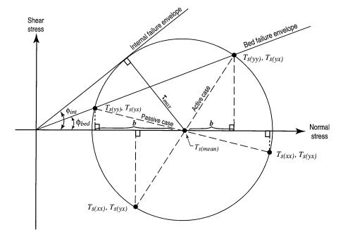
**Figure C1.** Mohr stress circle and Coulomb failure envelopes for a granular material that is simultaneously slipping along a bed and failing internally. The radius of the stress circle defines the maximum internal shear stress,  $\tau_{max}$ .
