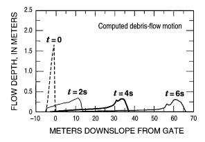
**Figure 24.** Predicted vertical cross-sectional profiles of the experimental debris flow of July 24, 1995. Profiles illustrate continuous acceleration and elongation of the debris flow surge during 6 s of motion down a uniform 31° slope. The profile of the static sediment heap denoted by t = 0 represents the initial condition. Vertical exaggeration is  $20 \times$ .
