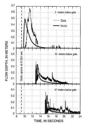
**Figure 25.** Comparison of measured and predicted flow depths as a function of time for the experimental debris flow of July 24, 1995. Predictions and data are shown for three cross sections, 2 m, 33 m, and 67 m downslope from the gate at the flume head. Flow commenced at the recorded time t = 9.324 s, and flow through all cross sections was on a uniform  $31^{\circ}$  slope.
