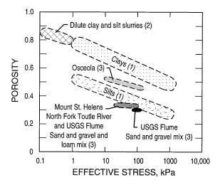
**Figure 20.** Data trends illustrating the approximate proportionality between fluid volume fraction (porosity) and the logarithm of effective stress in various soils and suspensions. Numbers identify data source: 1, *Lambe and Whitman* [1979]; 2, *Been and Sills* [1981]; 3, *Major* [1996].
