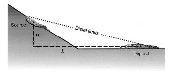
**Figure 2.** Schematic cross section defining H and L for debris flow paths. Strictly, H and L are defined by lines that connect the source area center of mass and the deposit center of mass. In practice, H and L are commonly estimated from the distal limits of the source area and deposit.
