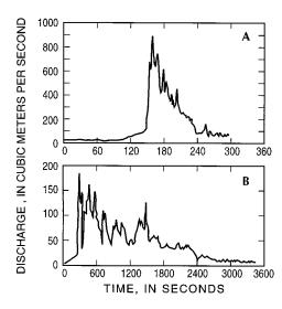
**Figure 9.** Measurements of debris flow discharge, which illustrate multiple surges within a flow event. (a) Data from Name River, Japan. (Redrafted from *Takahashi* [1991]; copyright A. A. Balkema). (b) Data from Chemolgan River, Kazakhstan [*Khegai et al.*, 1992].
