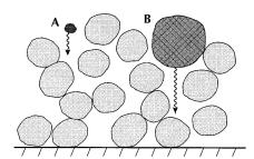
**Figure 7.** Schematic diagram illustrating the distinction between a small grain that remains suspended exclusively by viscous forces and thus can act as part of the fluid (grain A) and a large grain that requires interaction with other grains to remain suspended (grain B).
