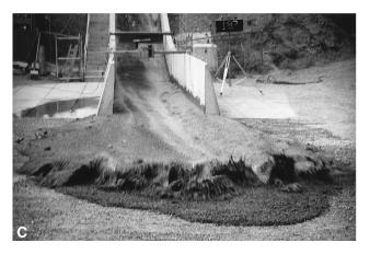
**Figure 8.** Photographs of advancing fronts of debris flow surges. (a) Nojiri River, Kagoshima, Japan, September 10, 1987. Flow is about 20 m wide and 2–3 m deep. (photo courtesy Japan Ministry of Construction.) (b) Jiang Jia Ravine, Yunnan, China, June 24, 1990. Flow is about 12 m wide and 2–3 m deep (photo courtesy K. M. Scott.) (c) USGS debris flow flume, July 20, 1994. Flow is about 4 m wide and 0.2 m deep.
