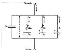
$$I = C_m \frac{dV_m}{dt} + \bar{g}_K n^4 (V_m - V_K) + \bar{g}_{Na} m^3 h (V_m - V_{Na}) + \bar{g}_l (V_m - V_l),$$
