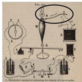
v. Helmholtz's method of estimating the velocity of a nerve pulse.
